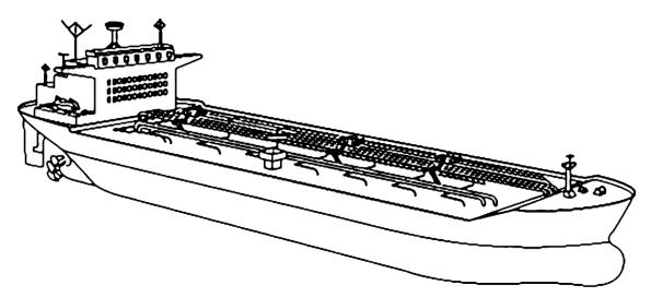
Distinguishing Features: The deck of a tanker is covered with pipes and pumps.
