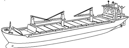
**Distinguishing Features:** Geared bulk carriers have cranes or derricks which allow them to discharge cargo in ports without shore-based equipment.
