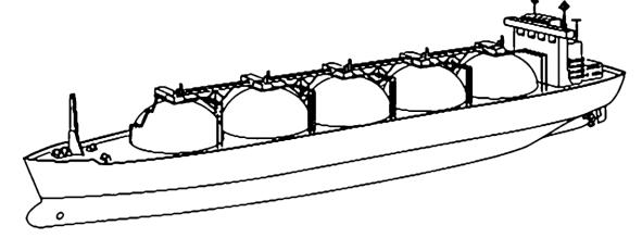
Distinguishing Features: spherical tanks half below and half above the deck.
