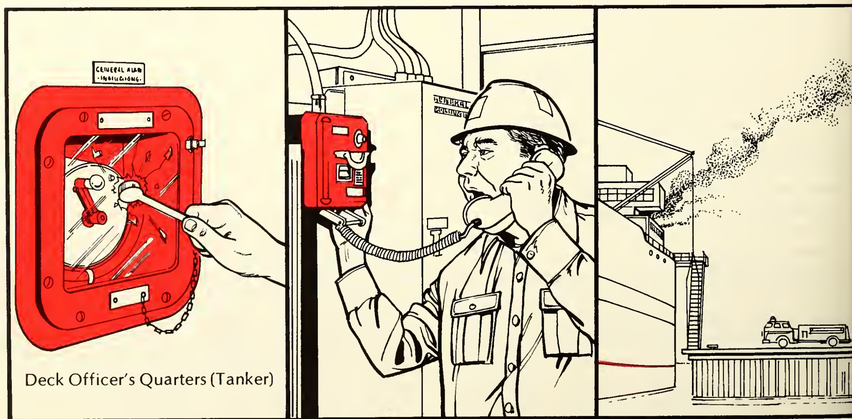
Figure 13.4. Crewmen must know how to (A) operate the ship's manual fire alarm system, (B) report a fire via the ship's telephone and (C) summon the land-based fire department when the ship is in port.
