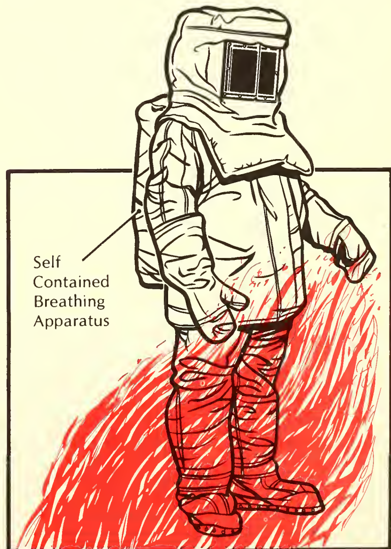
Figure 16.11. The entry suit allows the wearer to enter flames for a short time—the shorter the better. (Courtesy Fyrepel)
