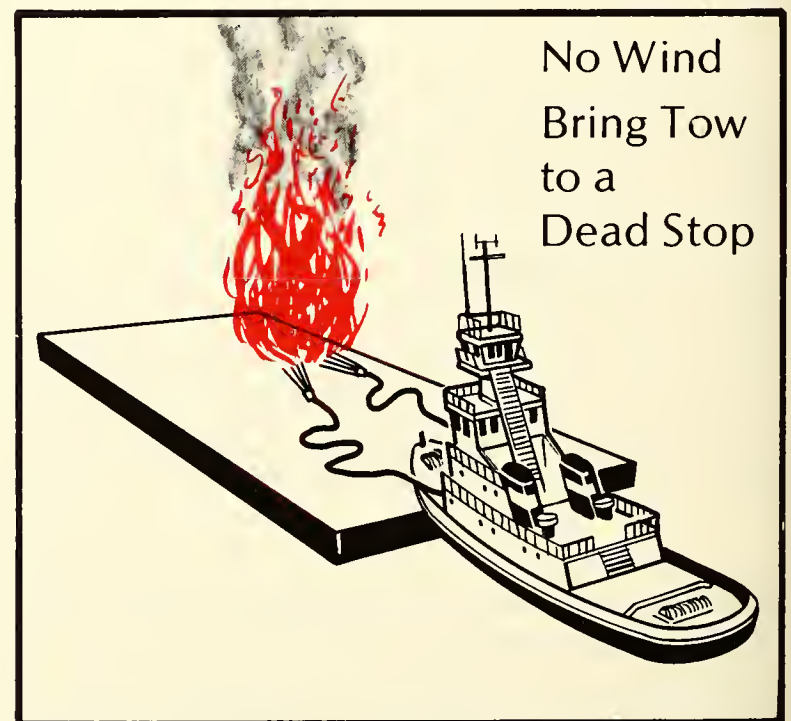
Figure 11.14. If there is no wind, the tug must be maneuvered to create a favorable air movement.
