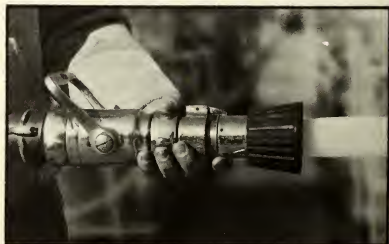
Figure 12.8. The adjustable fog nozzle can deliver a solid stream or two different fog patterns. A. The fully closed position. B. The fully open position with the stream selector set for a solid stream.
