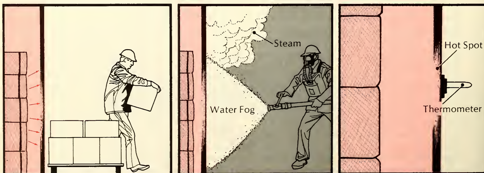
Figure 10.17. A. If possible, cargo should be moved away from hot bulkheads. B. Hot bulkheads may be cooled with water fog, applied until steam is no longer produced. C. Pyrometers are placed halfway between the deck and overhead.
