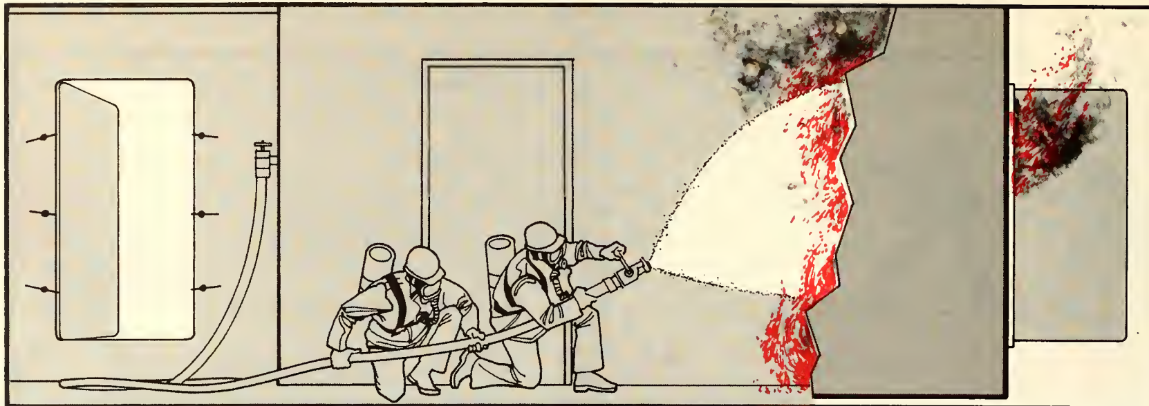
Figure 7.10. A high velocity fog stream can be used to drive heat and smoke ahead of firefighters when there is an outlet for these combustion products.
