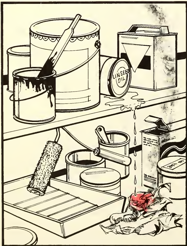
Figure 1.4. Careless disposal or storage of materials can lead to spontaneous ignition.
