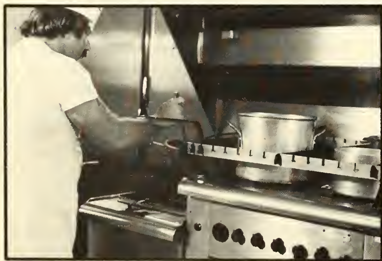
Figure 1.11. When underway, range battens should be used to keep pots from sliding off the cooking surface.
