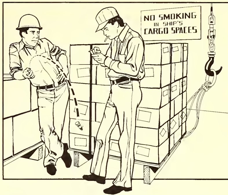
Figure 1.3. Smoking and careless disposal of smoking materials have caused many serious fires in cargo holds. Smoking must be prohibited in cargo spaces, and these spaces should be monitored during cargo handling.
